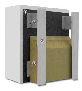
Structural Back-up Wall (by others): Steel or wood frame with glass mat gypsum sheathing in compliance with ASTM C1177, code compliant OSB or plywood sheathing, concrete or concrete masonry, existing structurally sound, uncoated brick or other masonry wall construction.
