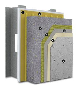
Substrate: Glass Mat Gypsum sheathing in compliance with ASTM C1177, Exterior or Exposure I wood-based sheathing (plywood or OSB), cement board in compliance with ASTM C1325, code compliant concrete, concrete masonry, portland cement plaster, or existing strucuturally sound, uncoated brick.
