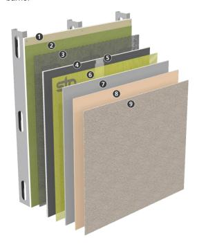
Substrate: Glass mat gypsum sheathing in compliance with ASTM C 1177, Exterior or Exposure 1 wood-based sheathing (plywood or OSB).
