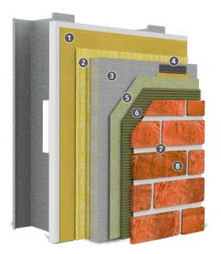
Substrate: Glass Mat Gypsum sheathing in compliance with ASTM C1177, code compliant wood-based sheathing (plywood or OSB)
