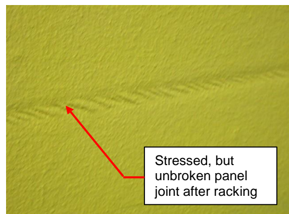
Figure 2: Panel joint waterproofing integrity of StoGuard is maintained after cyclic transverse loading, racking loads, and environmental cycling.
