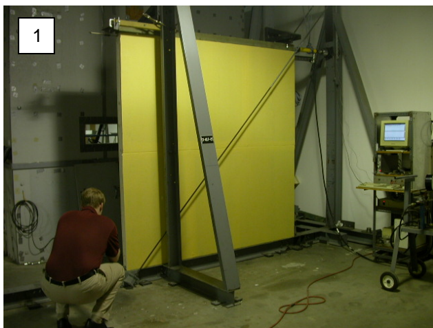
Photos 1 and 2: racking test set-up is depicted in photo 1 while joint under stress is depicted in photo 2. As with many of the tests identified in ICC AC 212 and the Canadian Technical Guides for air barriers and liquid applied WRBs (sheathing membranes), resistance to water penetration is evaluated after stress or fatigue tests.
