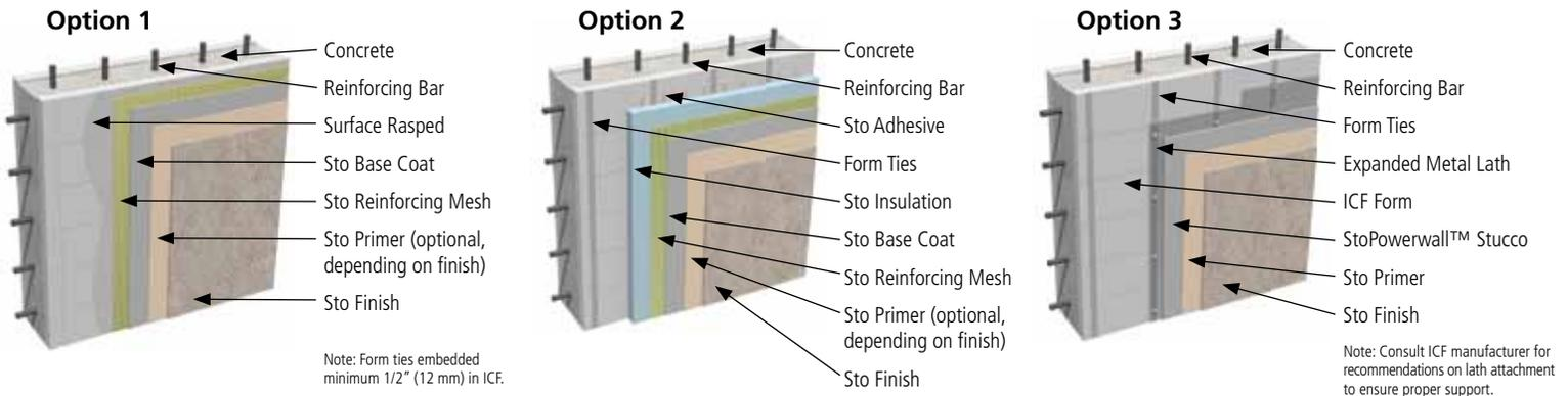
**Option 1: Coating System** Recommended when the walls are straight and flat with little leveling needed and ties are embedded at least 1/2 inch inside the ICF form.
