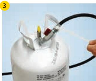
3 Verify the valve on the hose and the flow-control valve on the pistol are fully **CLOSED.** Secure hose to cylinder handle with plastic tie to protect hose and connection from incidental damage during use.
