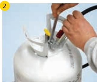
2 Hand-tighten hose fitting onto TurboStick cylinder. Avoid cross-threading the fittings which will result in leaks at the connection. Use properly sized open end wrench to tighten fitting. **DO NOT OVERTIGHTEN.**
