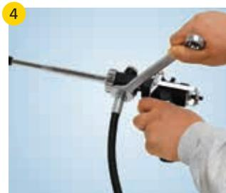
4 Hand-tighten hose fitting onto application pistol inlet fitting. **AVOID CROSS-THREADING.** Use properly sized open end wrench to tighten fitting. **DO NOT OVERTIGHTEN.**
