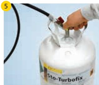
5 Open cylinder and hose valve. Observe for leaks. **DO NOT USE TOOLS TO OPEN OR CLOSE THE CYLINDER VALVE. CONTENTS OF CYLINDER ARE UNDER PRESSURE AND COULD CAUSE IN INJURY IF CYLINDER VALVE IS DAMAGED.**
