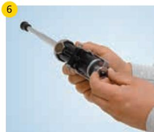
6 Open flow control valve on the back of pistol and dispense TurboStick material into an open container until steady flow and uniform consistency is achieved.
