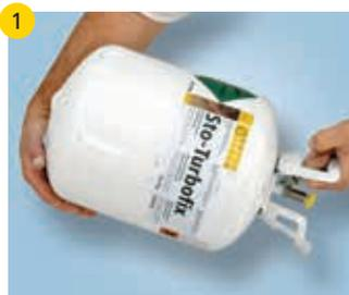
1 Hold cylinder horizontally and shake vigorously side-to-side for 10 to 15 seconds to mix contents.
