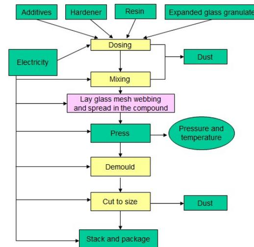
This method is specific to the manufacturing location. The product components are dosed and mixed. The glass fibre mesh is laid out in the press mould and the mixture distributed. After being pressed at an increased temperature, the carrier boards are demoulded and cut to size.
