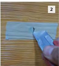
2 Place a piece of masking tape over the hole and trim out the hole with a sharp knife.
