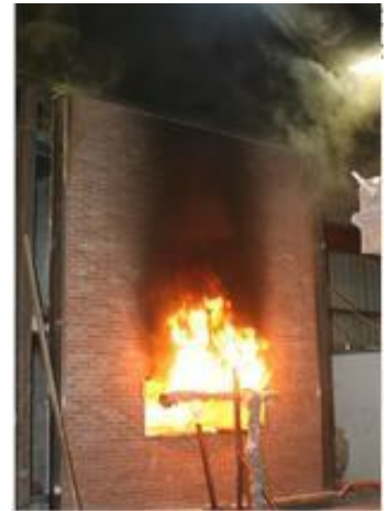
Photo 1. NFPA 285 testing of brick veneer cavity wall with foam plastic and a combustible WRB over steel frame construction
