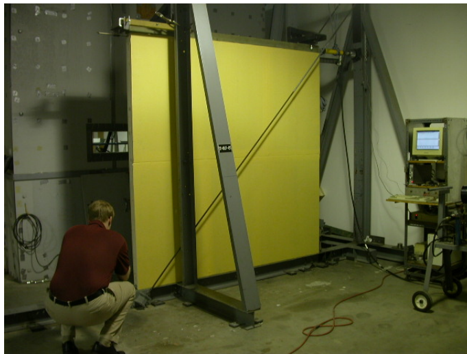
Figure 5. Racking test set-up in laboratory.
