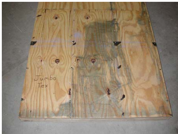
Figure 13. Building paper panel after ASTM E 331 water spray testing. Dye stains indicate source points and extent of leakage.
